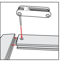
**Extrusion & Lock Connection**
